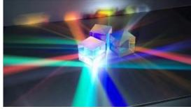
A trichroic prism splits light into three beams of light with different wavelengths (or colors). These prisms are used in some video cameras to send different colors of light to different color sensors. The prisms are coated with special coatings to filter and transmit different wavelengths of light. Click on the picture to view a video of the beautiful light produced by the prism. Students can complete a <u>See Think Wonder Template</u> after watching the video.
